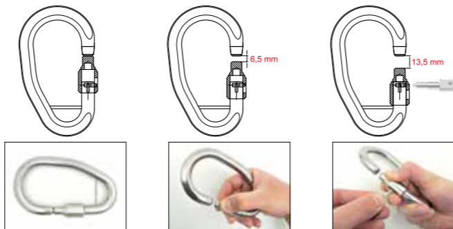
REST POSITION closed gate MANUAL OPENING for passing through the plates EMERGENCY OPENING WITH KEY for evacuation from safety line
